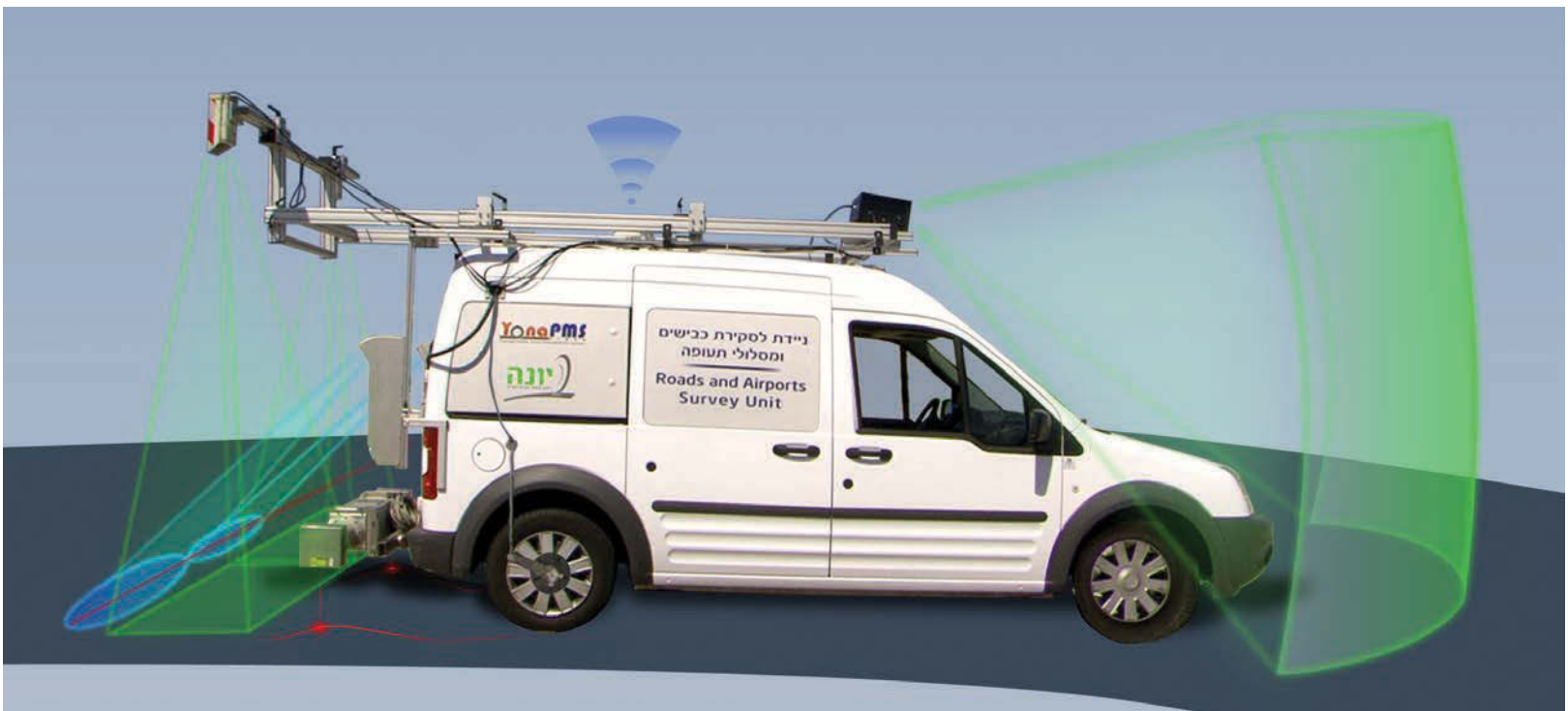
Non-dedicated vehicle, mounted with field data collection tools
